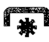
ATTACHMENT CLUTCH DISENGAGED
