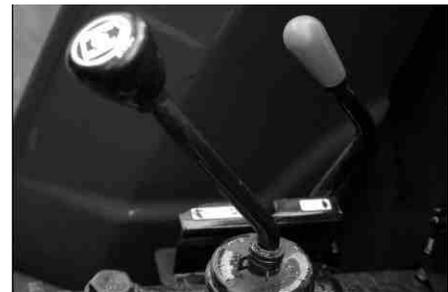
**NOTE:** When traveling downhill always remain in gear. Never declutch. The gear selected should be same as would be used to climb. For engaging/disengaging gear always depress the clutch
