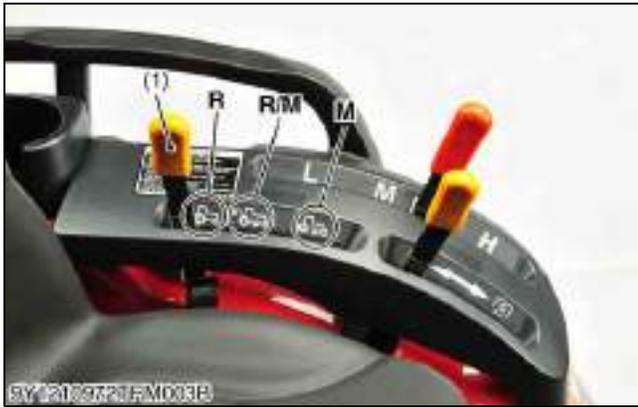
The PTO shift lever (1) is located at left side fender. The PTO shift lever (1) and the PTO shift arm (2) are linked with the control rod (3).
