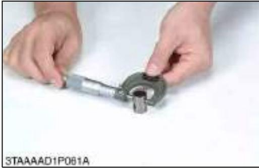
**Oil Clearance between Tappet and Tappet Guide Bore**
