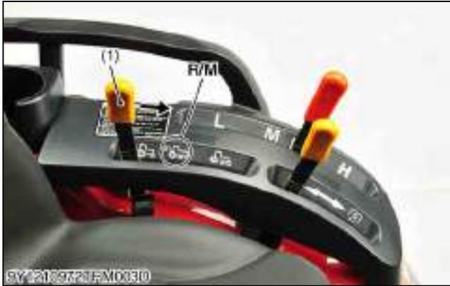
When the PTO shift lever (1) is set to "Rear PTO / Mid PTO" (R/M) position, the PTO shift lever (1) pulls the control rod.
