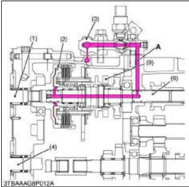
Independent PTO clutch (2) is located behind the HST pump shaft (1) in the transmission case.
