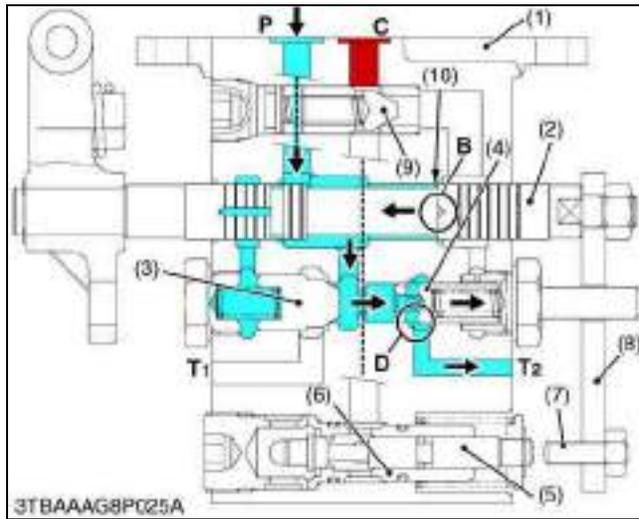
**Shockless mechanism operating (Lift to Neutral)**
