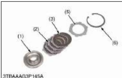
**PTO Clutch Discs and Brake**
