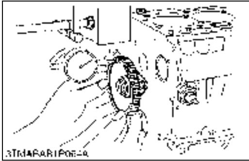
**Idle Gear 1 and 2 Side Clearance**
