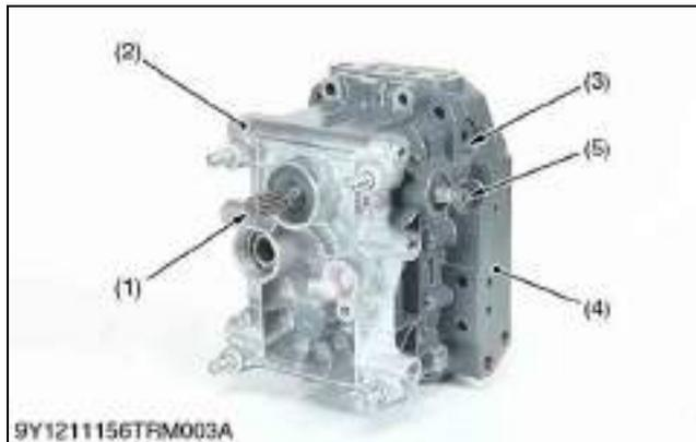
Hydrostatic transmission consists of variable displacement piston pump, fixed displacement piston motor and valve system.
