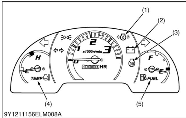
If the warning lamps of the Easy Checker™ come on during operation, immediately stop the engine, and find the cause as shown below.
