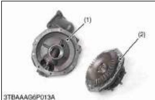
**Front Gear Case and Axle Flange**
