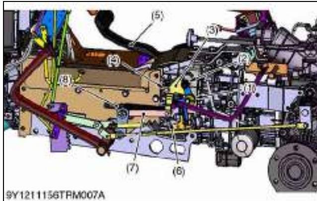
The HST pedal (5) and trunnion shaft (4) of swashplate are linked with the HST plate (7) and the neutral holder (3). As the front footrest of the pedal is depressed, the swashplate rotates and forward traveling speed increases. Depressing the rear footrest increases reverse traveling speed.
