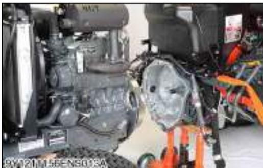
**Separating Engine from Front Axle Frame**
