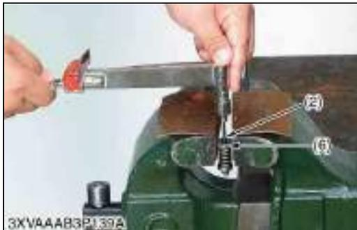
**Readjustment of Relief Valve (When the HST does not work due to its loose hexagon socket head screw)**
