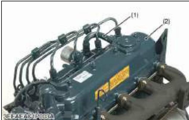
Closed breather system has been adopted to prevent the release of blow-by gas into the atmosphere.
