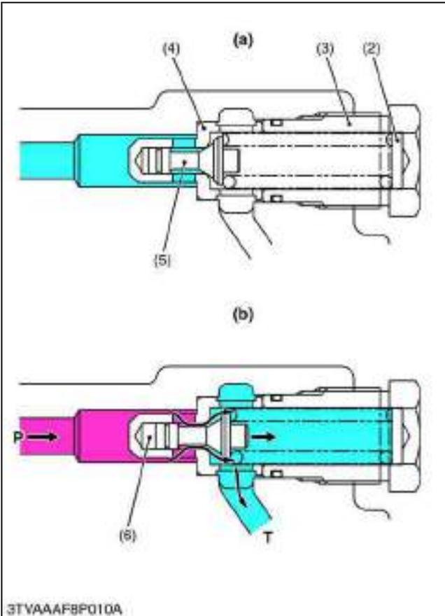
The hydraulic raising and lowering circuit is fitted with a relief valve to control the maximum pressure.
