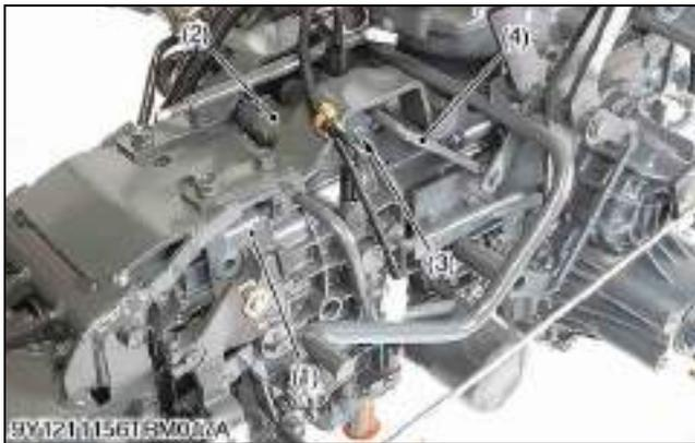
Independent PTO control valve (2) is located at transmission case (1).
