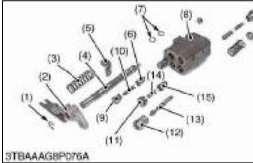
**Disassembling Position Control Valve**
