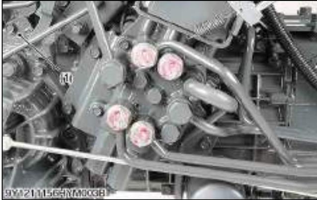
The hydraulic block type outlet is located at the right hand side of the engine.
