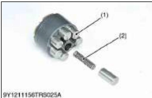
**Cylinder Block Bore and Pistons**
