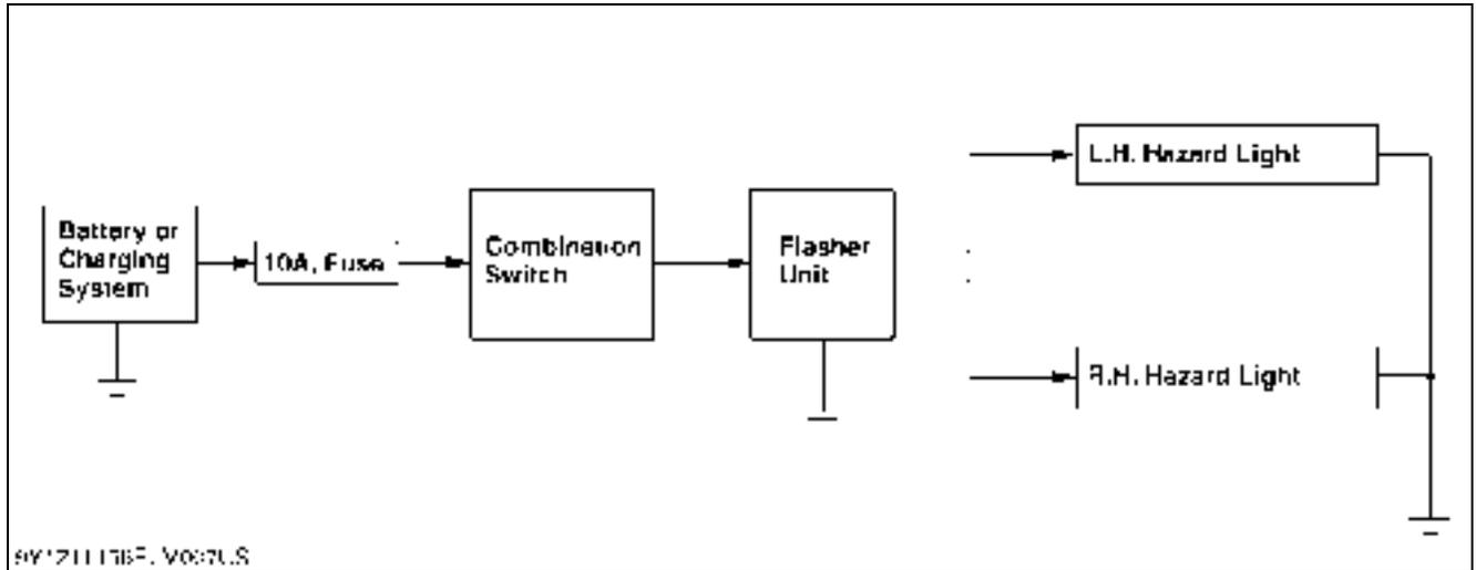
Hazard switch has two positions; **ON** and **OFF**. Blinking the hazard lights as shown in the figure above. The hazard light is operative when the key switch is in either the **ON** or **OFF** positions.
