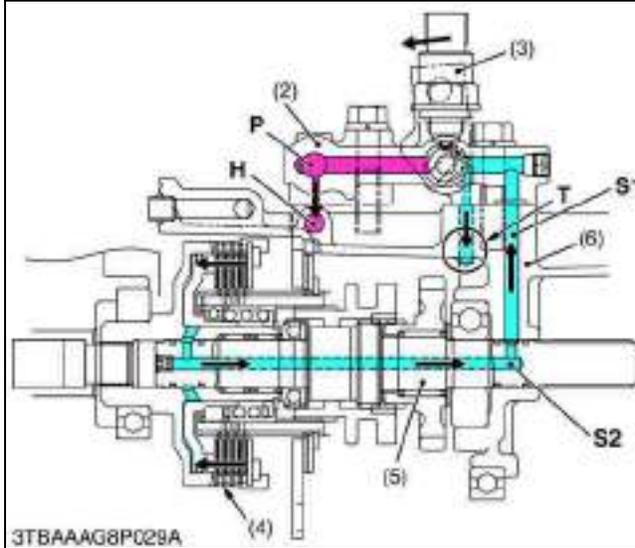
When the independent PTO lever (1) is shifted to the "DISENGAGED" position, the PTO arm (3) is turned to "OFF" position.
