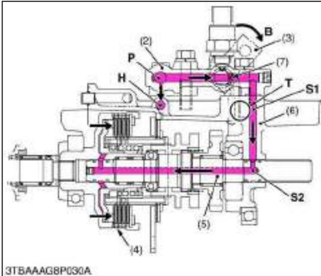
When the independent PTO lever (1) is shifted to the "ENGAGED" position, the PTO arm (3) is turned to "ON" position.
