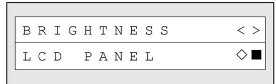
4. Press the (◇) of monitor panel mode selector switch 1. The screen will change to the display shown on the right and it will be possible to adjust the brightness.
