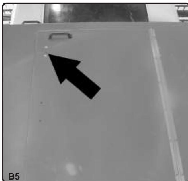
Open the cover above the engine compartment like this:
