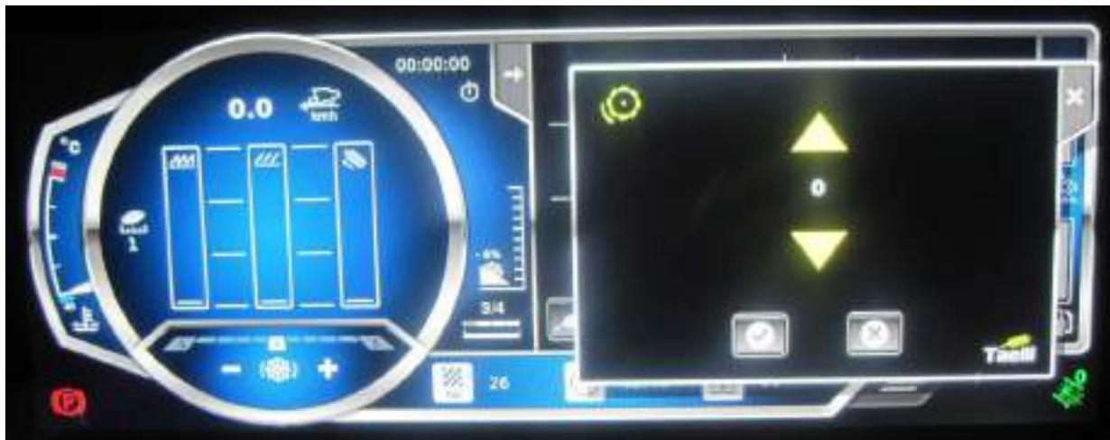
When pressing grain crop symbol at **Harvesting adjustments** window, “Taelli”- control system (OPTION) will pop-up. On this window you can make proper adjustments for different crops and then moving between them becomes more easy.
