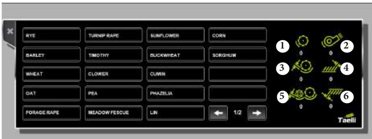
Pressing any meter on bottom of the home view will open a window which displays all meters. You can choose three meters to be displayed in home view simply by pressing desired meter.
