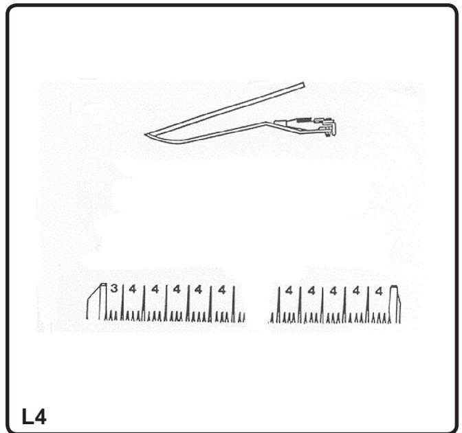
**CROP LIFTERS (fig. L4) Spaced Correctly.**
