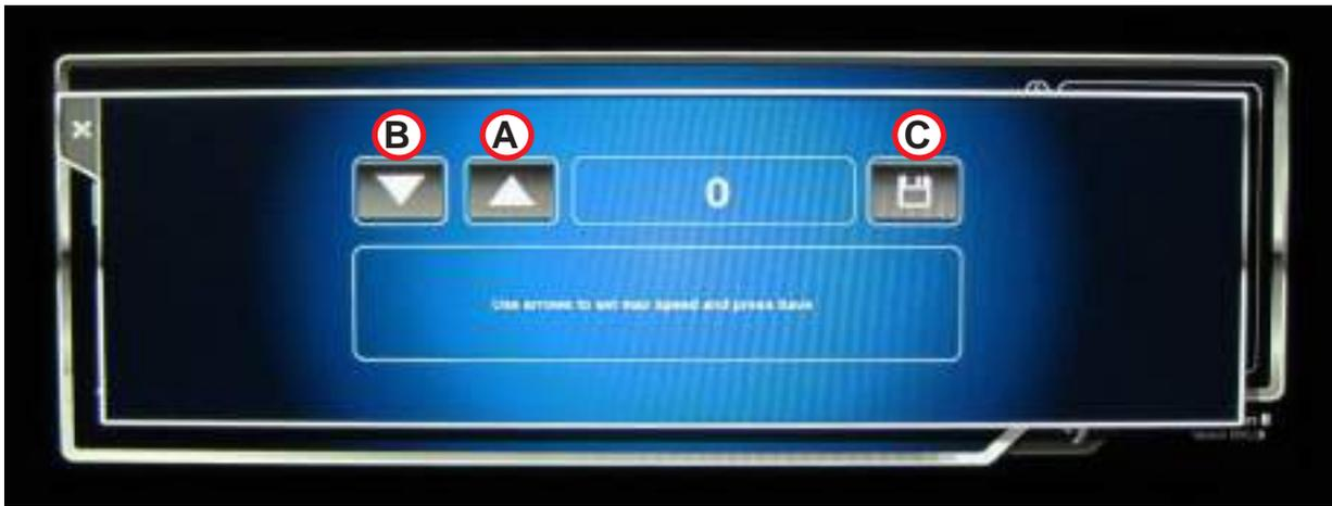
Push button (A) until fan speed doesn't raise anymore. Lower speed 50 units with (B) button. Save calibration value with (C) button.
