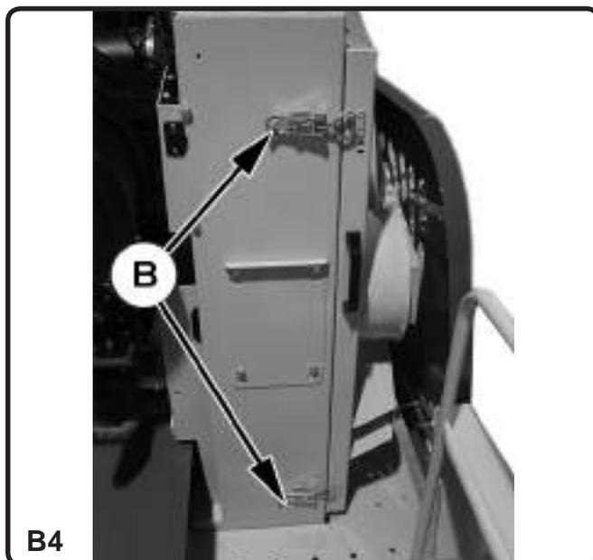
Open the locking on the grain tank cover, fig. B5, by placing the tool in the hole and turning counter-clockwise.
