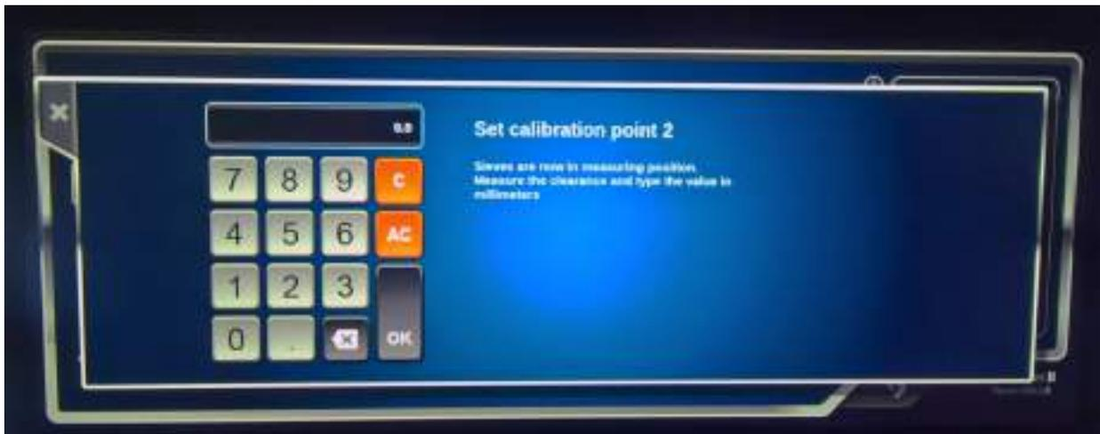
When keyboard pops-up again you have to measure the lower sieve opening clearance and input the 2nd value. Accept with OK button.
