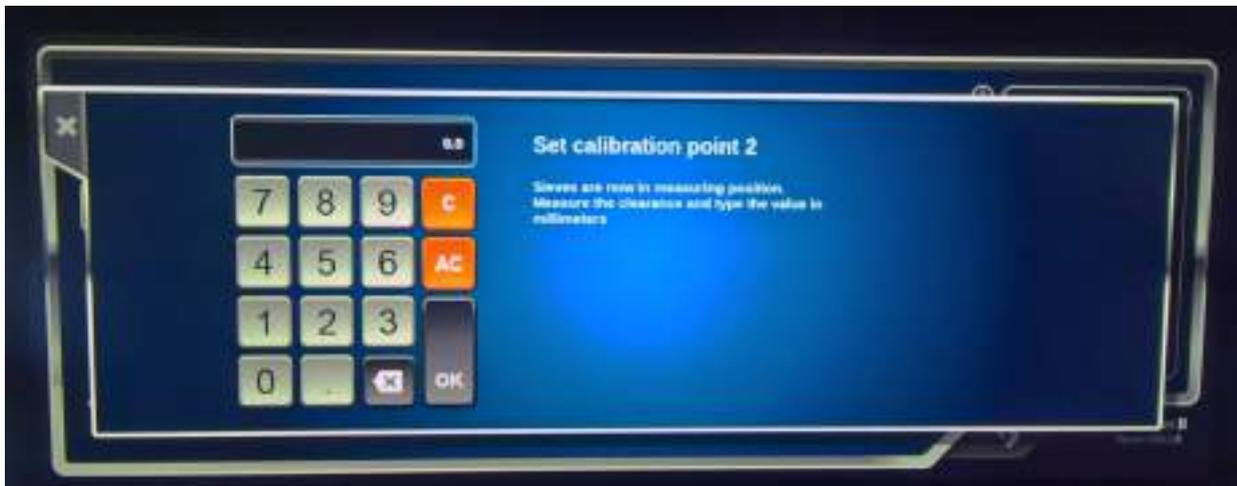
When keyboard pops-up again you have to measure the upper sieve opening clearance and input the 2nd value. Accept with OK button.
