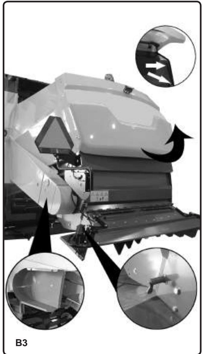
To clean the equipment, the fan unit in front of the radiator may be turned open by opening latches B. (Fig.B4)
