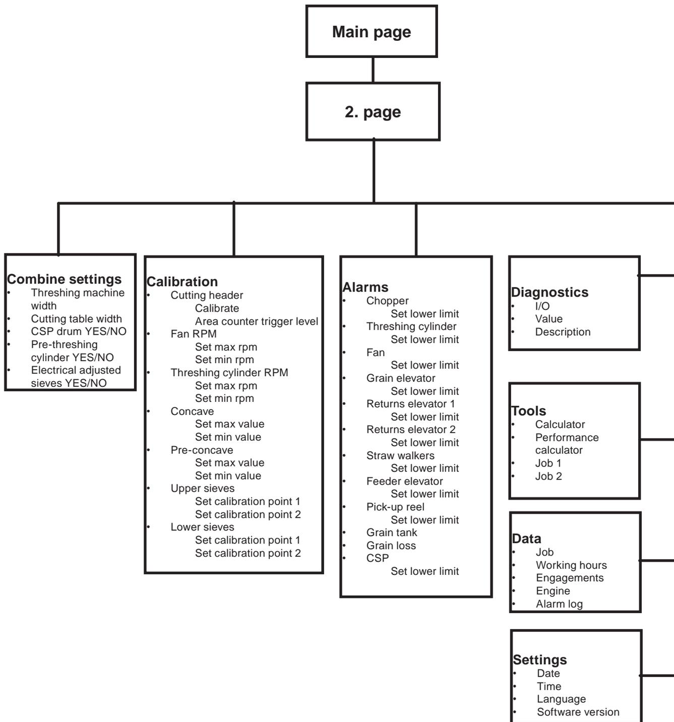
2. **page** button at the main page opens a menu for settings, calibration, adjusting alarms, diagnostics, tools for harvesting and data menus.
