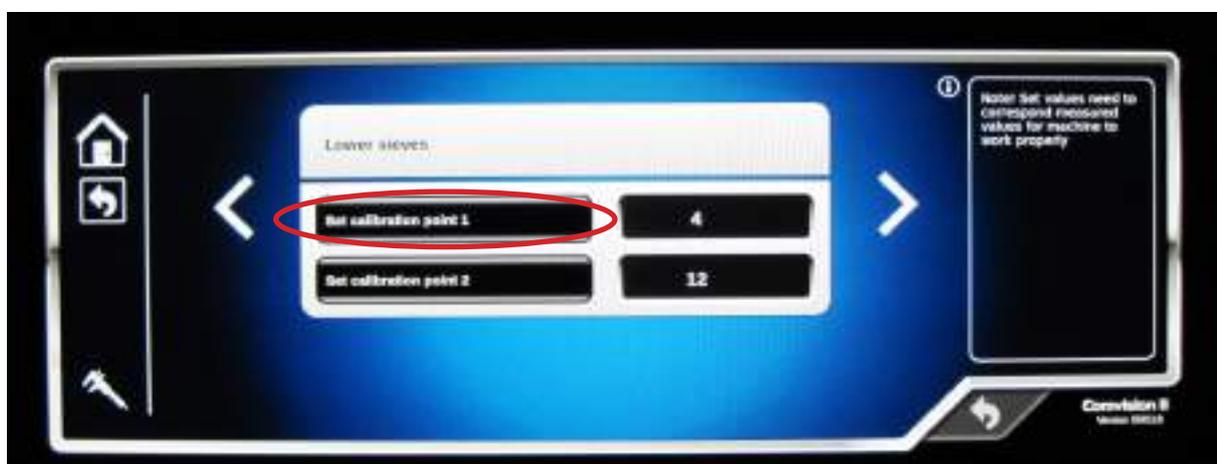
Operating actuator runs lower sieve to open and close positions automatically. And automatically calibrates those values.
