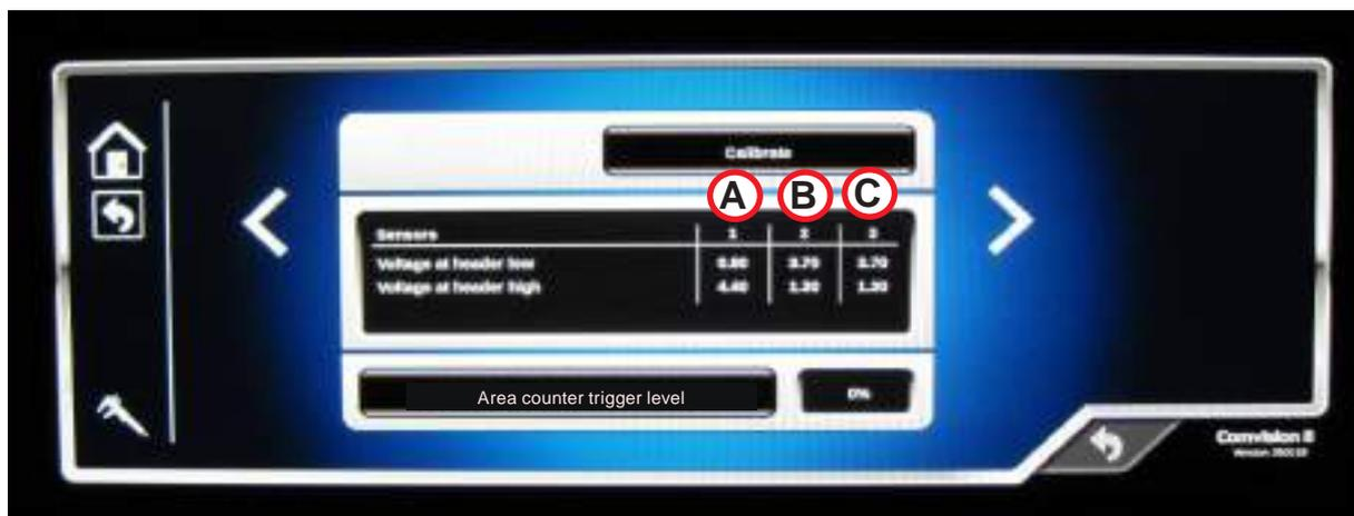
After calibration you can see the calibration values in columns. (A) Feeder house sensor. (B) Left hand side AHC sensor. (C) Right hand side AHC sensor. Values are Voltage values from sensors to cabin control unit when cutting header is down against ground and maximum up position.
