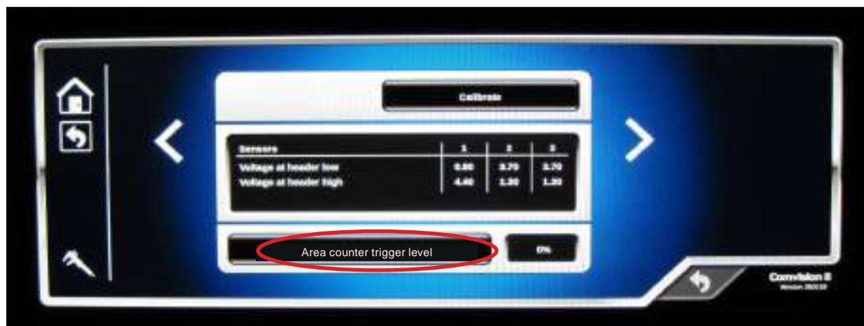
Adjust cutting header to height which you want hectare counter to activate/deactivate and push "save" button.
