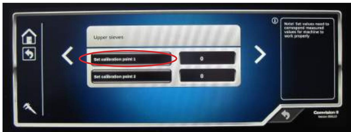
Operating actuator runs upper sieve to open and close positions automatically. And automatically calibrates those values.
