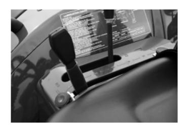
FIG.2-27 position control lever
