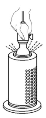
FIG.3-12 Element check https://www.tractormanualpdf.info/
