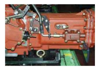
Fig.5-33 Main shift lever linkage
