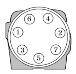
Align the marks made in STEP 2,and install the end cap. Install and evenly tighten the torx hand screws in two stages to a torque of 17 Nm(12 lb ft) then to 25 to 30 Nm (19 to 22lb ft) in the sequence shown.
