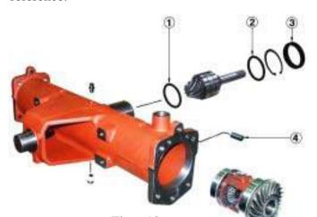
6) Remove the bearings from the Axle housing And the ring gear, and then the ring gear can be separated from the Axle housing.
