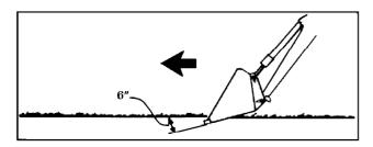
With the bucket level, start a cut at the notch approximately 2" deep.
