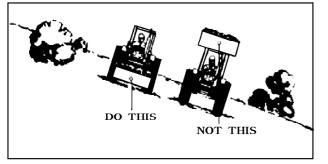
When transporting the load,Keep the bucket as low as possible to avoid tipping,in case a wheel drops in a rut.
