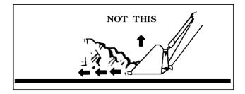
Note: Do not be concerned if the bucket is not completely filled during each pass Maximum productivity is determined by the amount of material loaded in a given period of time. Time is lost if two or more attempts are made to fill the bucket on each pass
