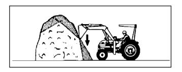
If the pile sides are too high and liable to cause cave-in, Use the loader to break down the sides until a slot can be cut over the top.
