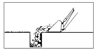
Leave dirt in the bucket because dumping on each pass wastes time.
