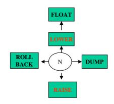
The single lever and joystick control lever is mounts on the tractor from the factory. The control lever has the safety lock function.
