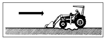
Backgrade occasionally with a loaded bucket to keep the working surface free of ruts and holes.Hold the lift control forward in FLOAT POSITION so the full weight of the bucket is scraping the ground.Use only the heel of the bucket while backgrading.
