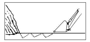
It is important to keep the bucket level when approaching a bank or pile. This will help to prevent gouging the work area
