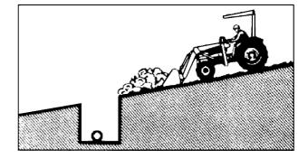
Operate at right angles to the ditch, Take as big as the tractor can handle without lugging down.
