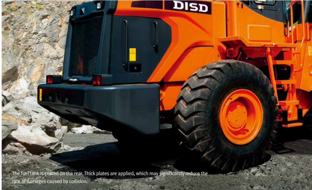
The fuel tank is placed on the rear. Thick plates are applied, which may significantly reduce the rate of damages caused by collision.
