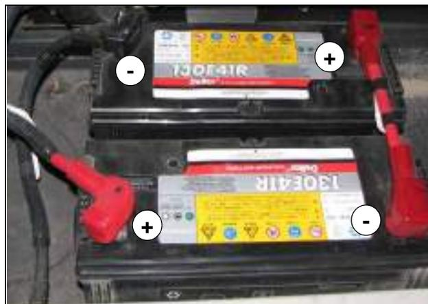
3. Connect the cable (positive terminals), the cable (negative terminal) then install the terminal sleeves.
