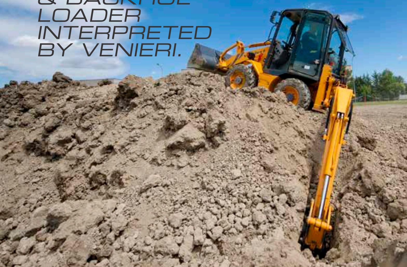
The compact 4x4x4 VF 1.33B loader & backhoe loader has reached the goal to work as a skid loader or as a mini-excavator, but overcoming the limits of the single skid loader and of the single mini-excavator.
